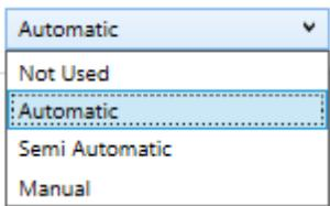
This setting gives the tuner options on how he would like to set up the tiptronic operation and LED indication for each Map. This is useful for modes like towing, racing and low range. If it is used as automatic only without buttons, select Not used. These modes may be set up differently for each of the 4 maps.
